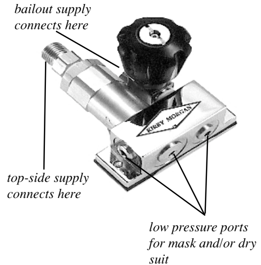
Attachment points for the DSI Manifold Blocks
