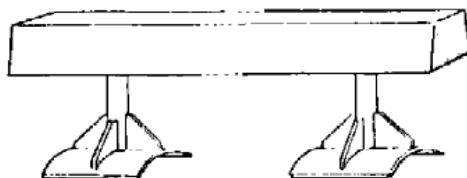
5. Tubular stand-off arms from anode body with gussets and double plate.
