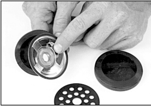
Fig. 6.13 Inspect the mylar cones.
