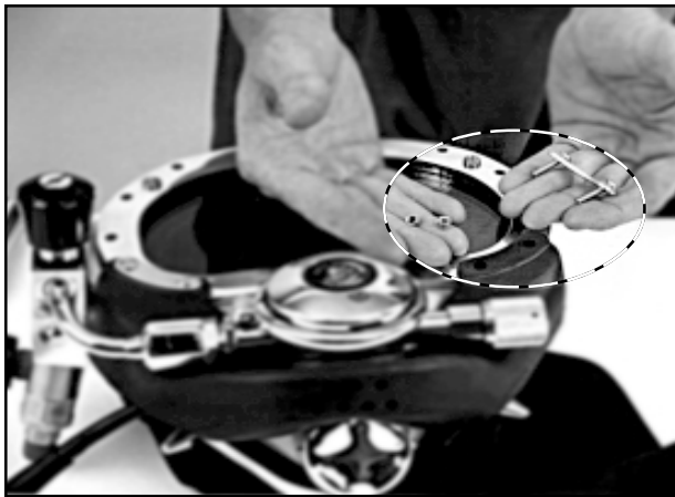
Fig. 6.5 Don't lose the whisker spacers.
