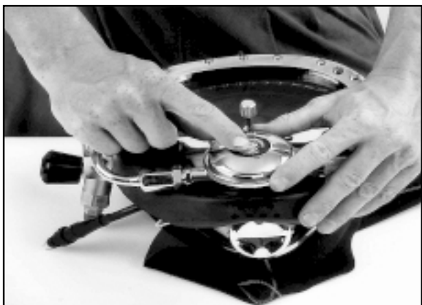
Fig. 5.25 Pressing the purge button.
