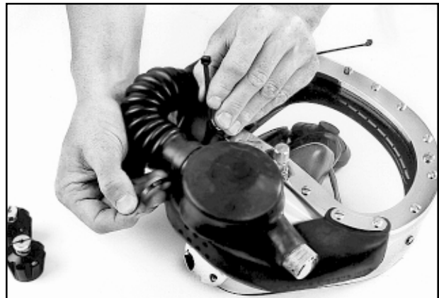
Fig. 7.5 Attach the tie wraps.
