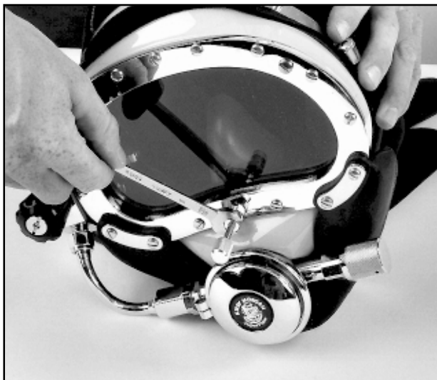
Fig. 5.8 Unscrew the nose block packing nut.
