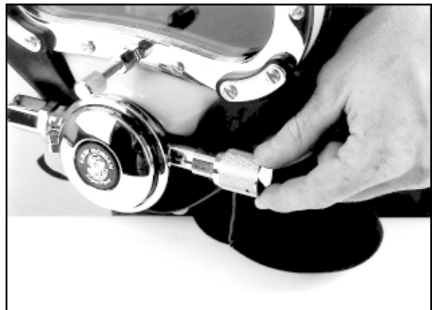
Fig. 6.65 The adjustment knob must turn freely.
