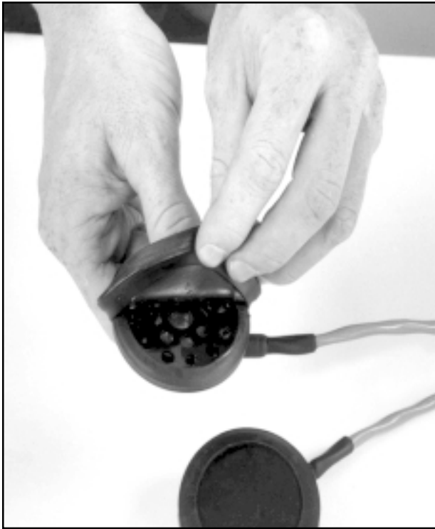
Fig. 5.4 Remove the earphone covers so the earphones can dry completely.
