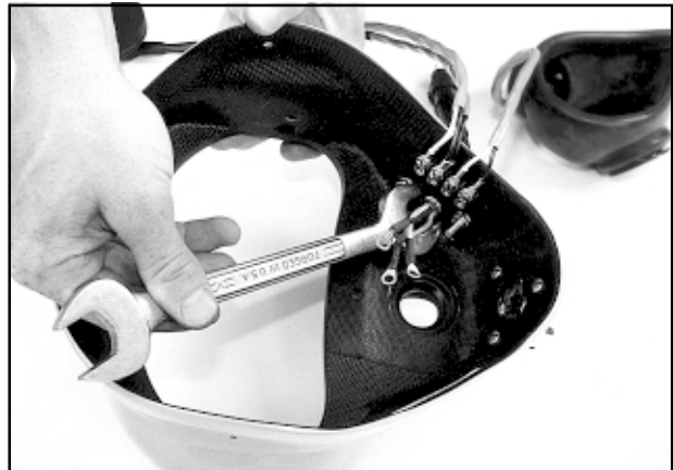
Fig. 6.19 Tighten the nut on the packing gland.
