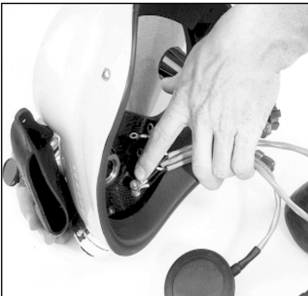
Fig. 6.14 Remove the nut from the communications posts.
