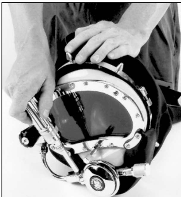
Fig. 5.14 Remove the regulator clamp screw.
