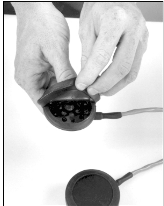
Fig. 6.12 Removing the rubber cover from the earphone.
