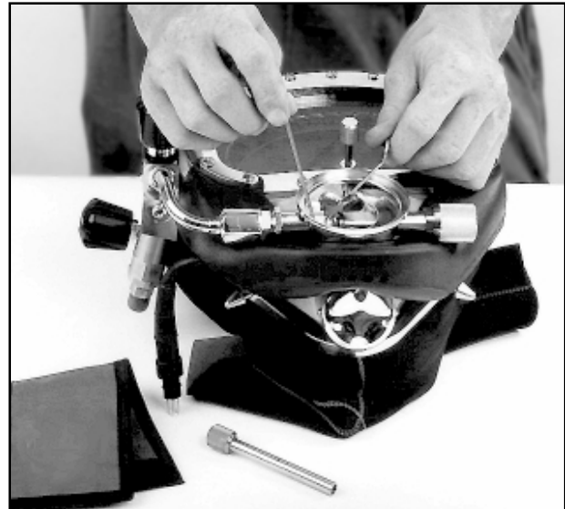
Fig. 5.23 Using the DSI Regulator Adjustment tools.
