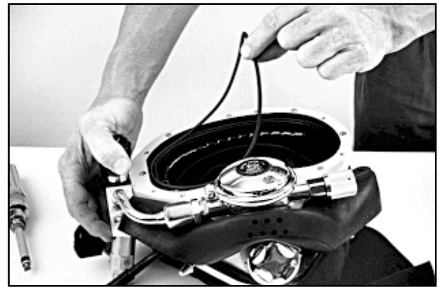
Fig. 6.7 Install the port O-ring .
