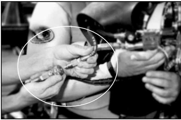
Fig. 2.13 The use of a quick disconnect fitting makes diving operations easier.
