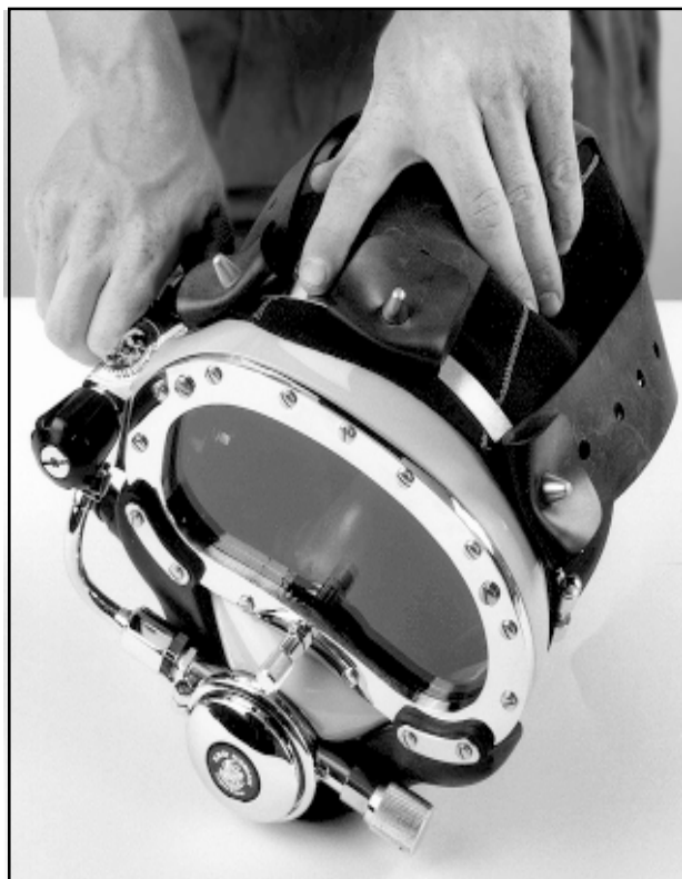
Fig. 5.7 The hood should protrude a minimum from 1/4 to 1/2 inch from under the bands.
