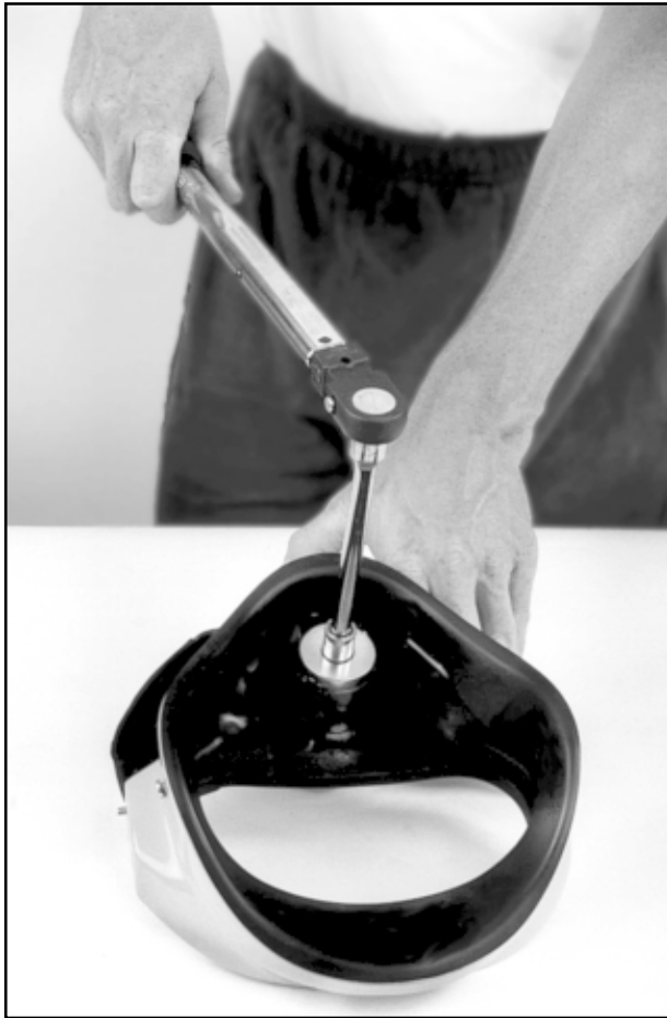
Fig. 6.59 Use the proper socket to remove the regulator mount nut.
