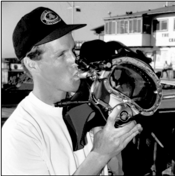
Fig. 2.3 Always check the one-way valve prior to diving.
