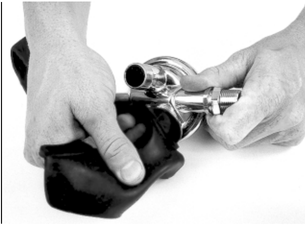
Fig. 6.51 Removing the whisker from the regulator.
