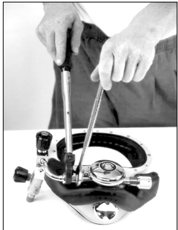
Fig. 6.47 Tightening the jam nut.
