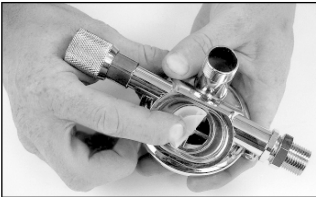
Fig. 6.52 Inspecting the regulator exhaust.
