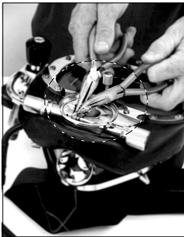
Fig. 5.26 Bending the lever up.
