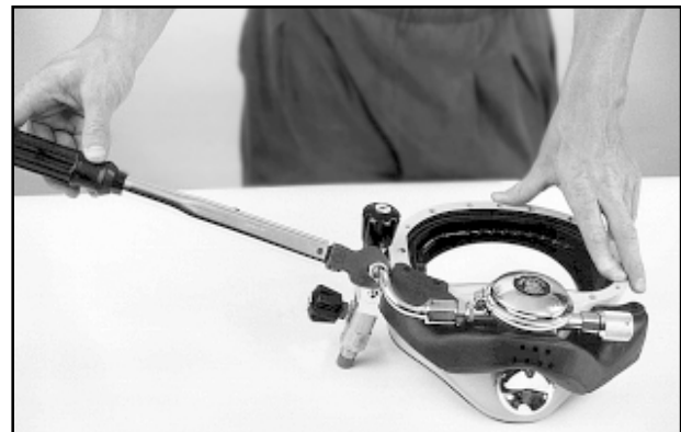
Fig. 6.22 Disconnect the bent tube assembly from the sideblock.
