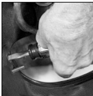
Fig. 6.28 Remove the alignment screw.
