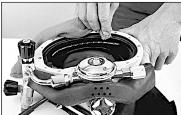
Fig. 6.6 Clean the O-ring groove.
