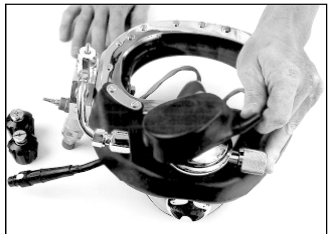
Fig. 7.2 Install the regulator cover.
