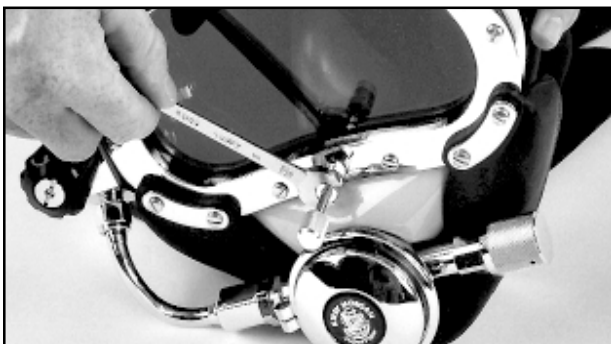
Fig. 6.3 Remove the nose block packing nut.
