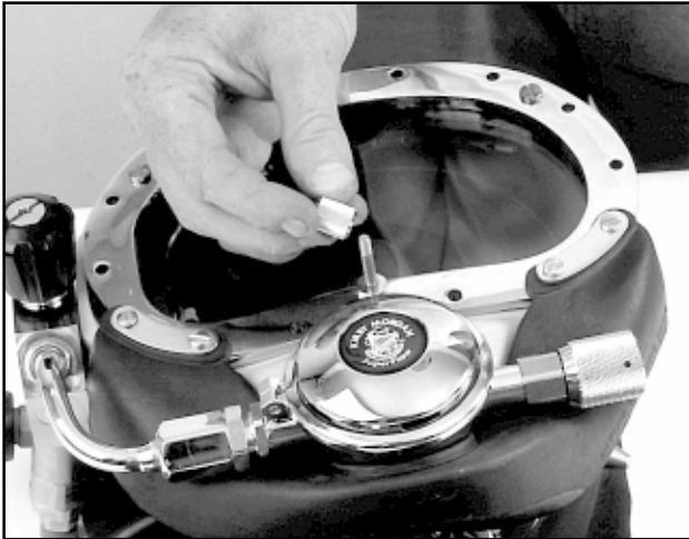
Fig. 6.2 Remove the nose block device knob.
