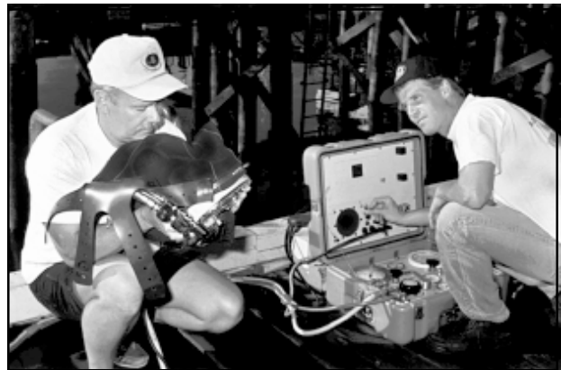
Fig. 2.8 Always check the communications with the mask prior to each dive.
