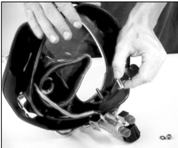
Fig. 6.27 The air train standoff on the KMB 28.
