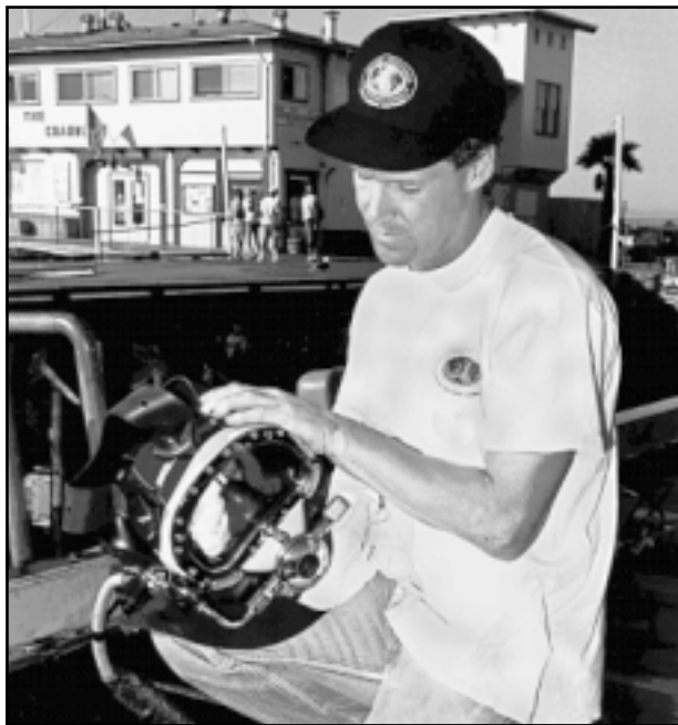
Fig. 2.1 Clean the face port prior to use.
