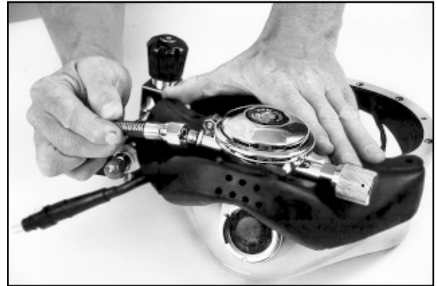
Fig. 6.42 Replacing an "A" regulator hose.
