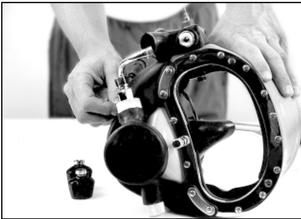
Fig. 7.4 Install the PVC flanges.
