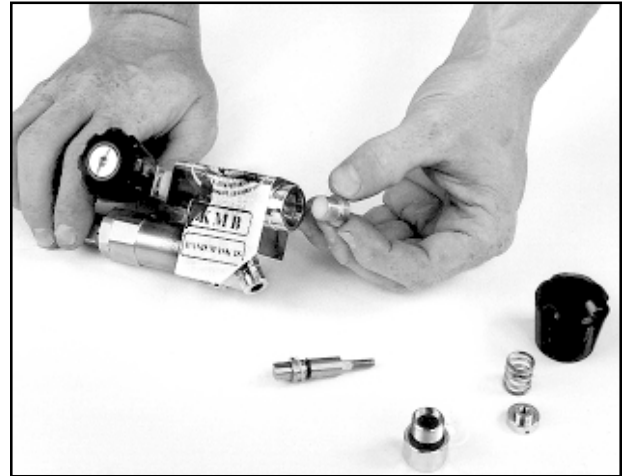
Fig. 6.36 The seat should be removed from the side block for inspection.
