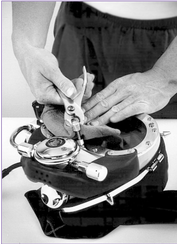
Fig. 6.11 Use a pair of pliers and a rag to tighten the nose block device knob.
