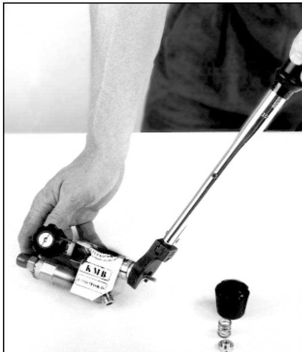
Fig. 6.35 Removal of the valve bonnet.
