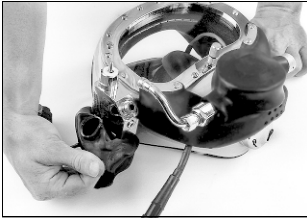
Fig. 7.3 Install the side block cover.
