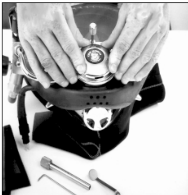
Fig. 5.24 Push down tightly on the cover.
