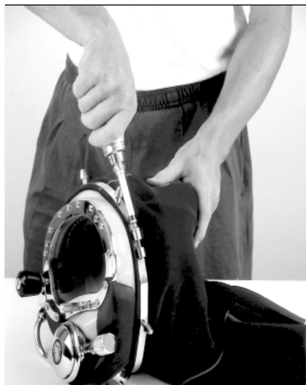
Fig. 5.3 Remove the hood by unscrewing the band screws.
