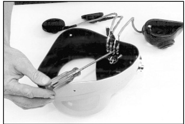
Fig. 6.16 Remove the earphone wire lugs from the terminal block.
