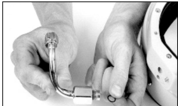
Fig. 6.45 Replace the O-ring on the bent tube if it is worn.
