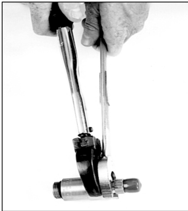
Fig. 5.10 If no vise is available you may use two wrenches to disassemble the valve.
