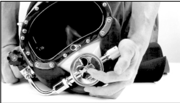
Fig. 5.22 Checking the play in the lever.
