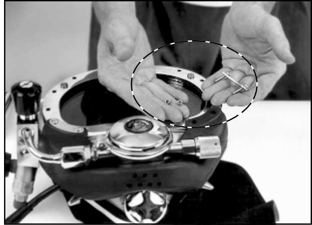
Fig. 6.53 Make sure the whisker spacers are in position.
