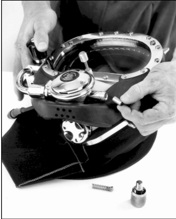
Fig. 5.19 Install the piston in the regulator.
