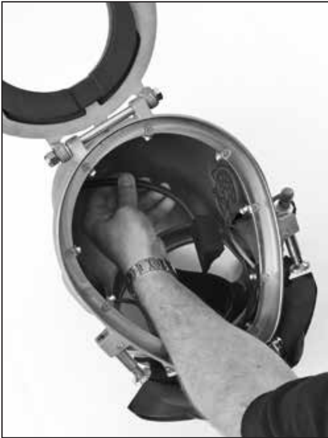
Remove the air train with the air train body.
