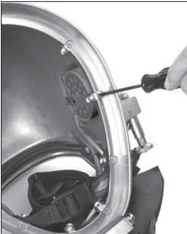
Removing the snap tab that also holds the earphone retainer.
