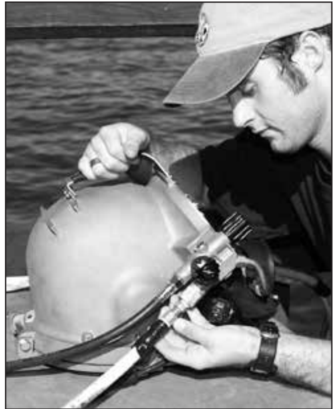
Connecting the umbilical to the helmet.
