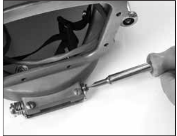
Remove the screw from the port side of the swing tongue catch.
