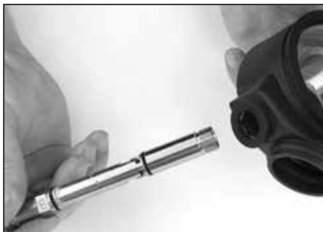
You can remove the main tube if it needs attention.
