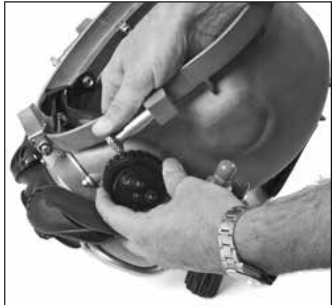
The nut must be securely fastened to hold the com module in position. Hand tighten only.
