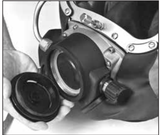
Remove the regulator cover to inspect the diaphragm.
