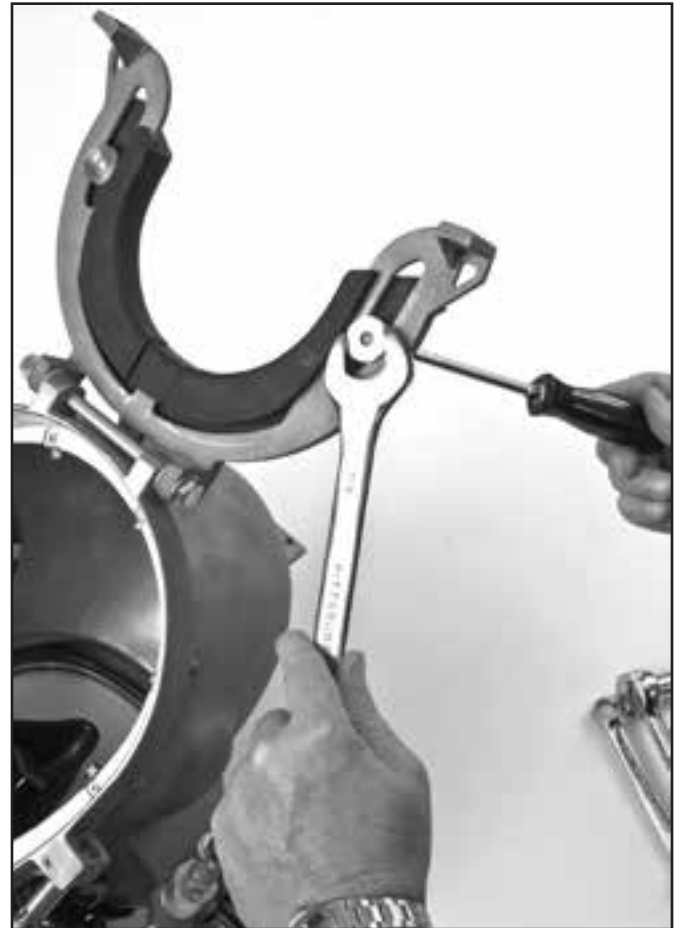
Unscrew the two screws that hold the neck pad.
