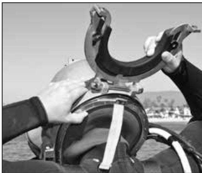
Push the neck dam/ring up into the neck ring on the base of the helmet .
