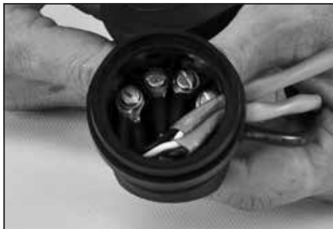
Installing the left earphone wires.
