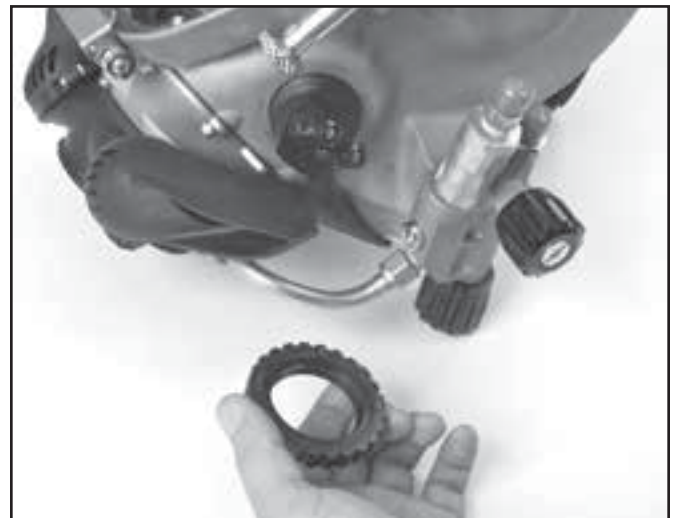
The large plastic nut is removed from the communications module.
