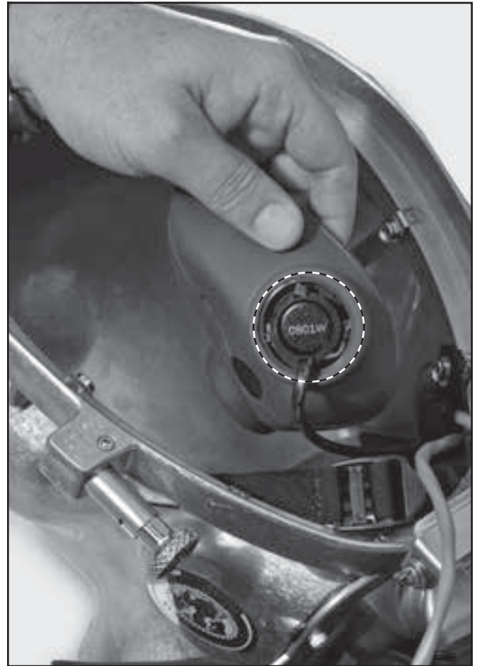
The microphone must be removed from the oral/nasal mask.
