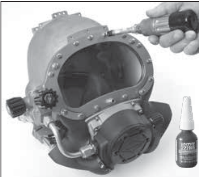
Always use a torque screwdriver to check the tension of the port retainer screws. Although the handle has been removed from this helmet, it is not necessary to remove the handle to remove the port retainer on the KM77.
