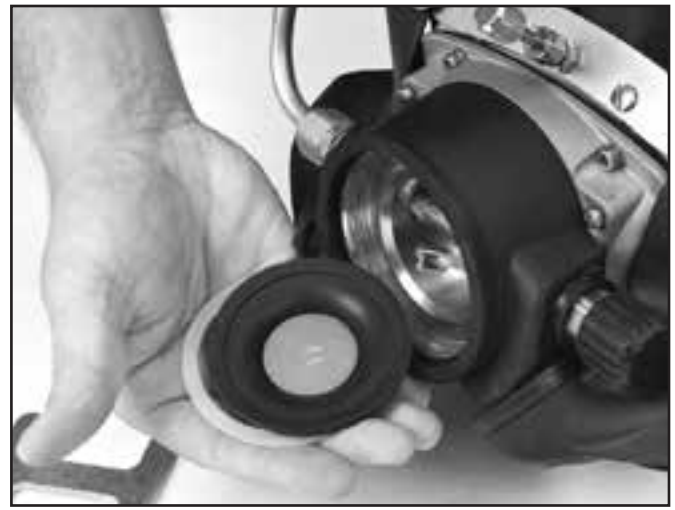
Remove the diaphragm and washer.
