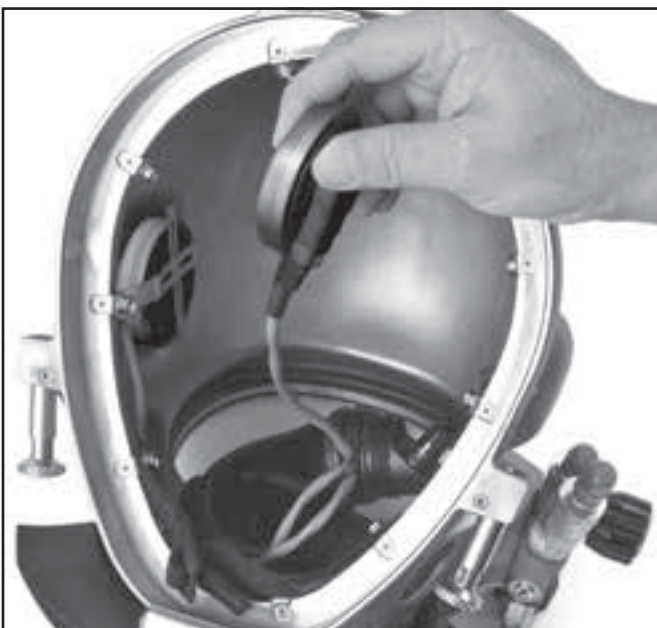
Remove the earphones from the earphone retainers.
