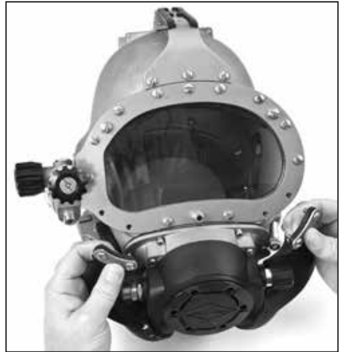
The whiskers are fastened to the face port using two screws on each side.
