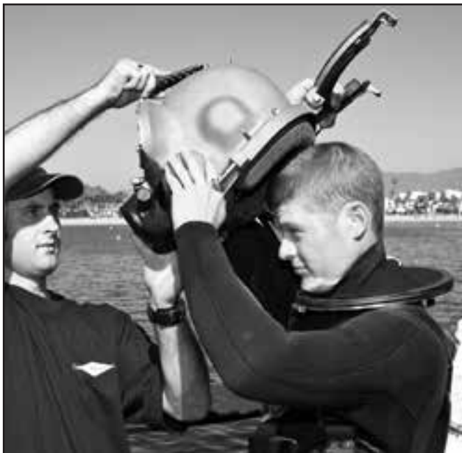
Open the locking collar/neck pad assembly fully.
