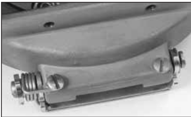
Properly assembled swing tongue catch.
