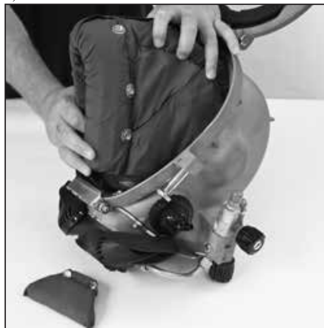
Removing the head cushion.
