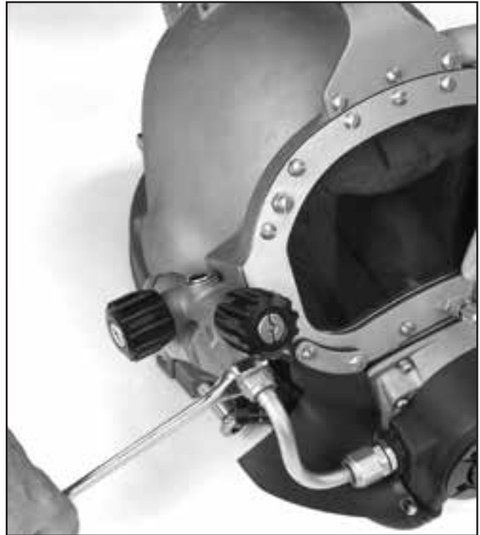
Loosening the bent tube from the side block.
