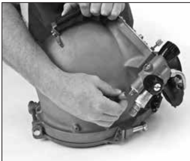
Cover the air inlet and emergency gas valve openings with dust caps when not in use.
