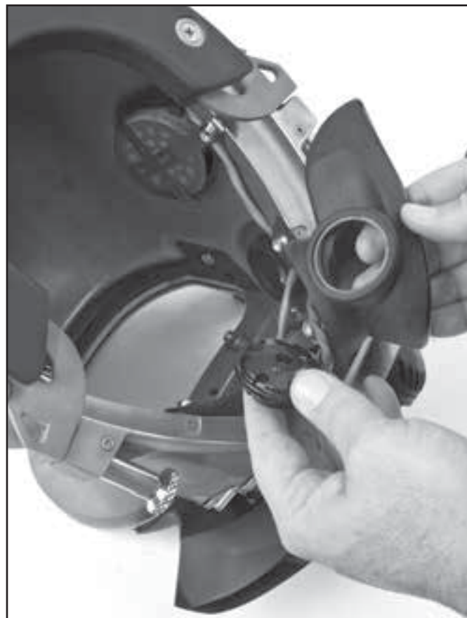
Install the microphone in the oral nasal mask.
