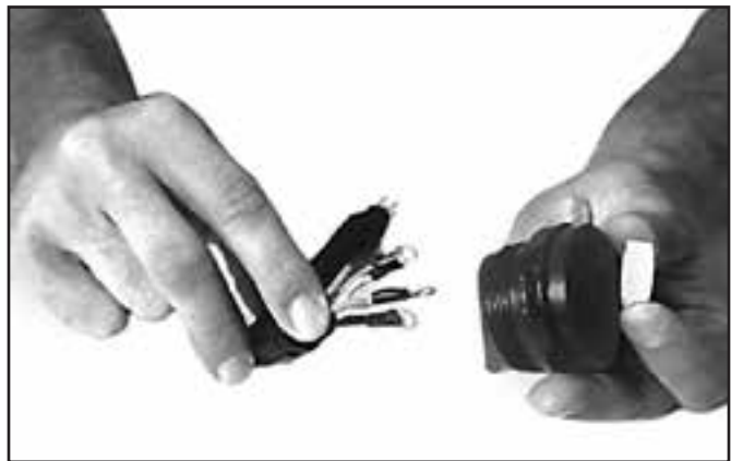
Pull the connector out of the module.
