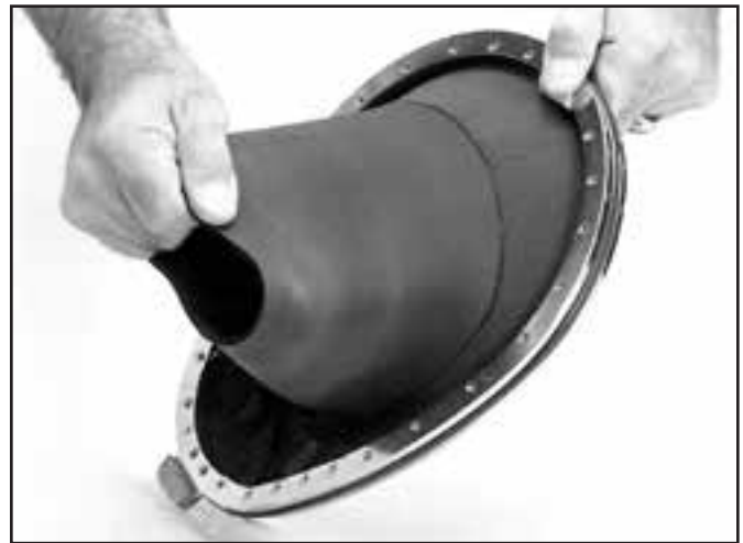
Check the neck dam for holes.
