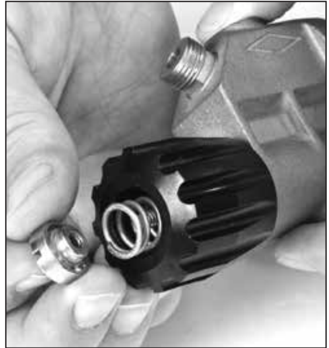
Remove the nut from the defogger valve knob.
