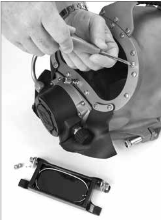
Remove the two plug screws from the port retainer.
