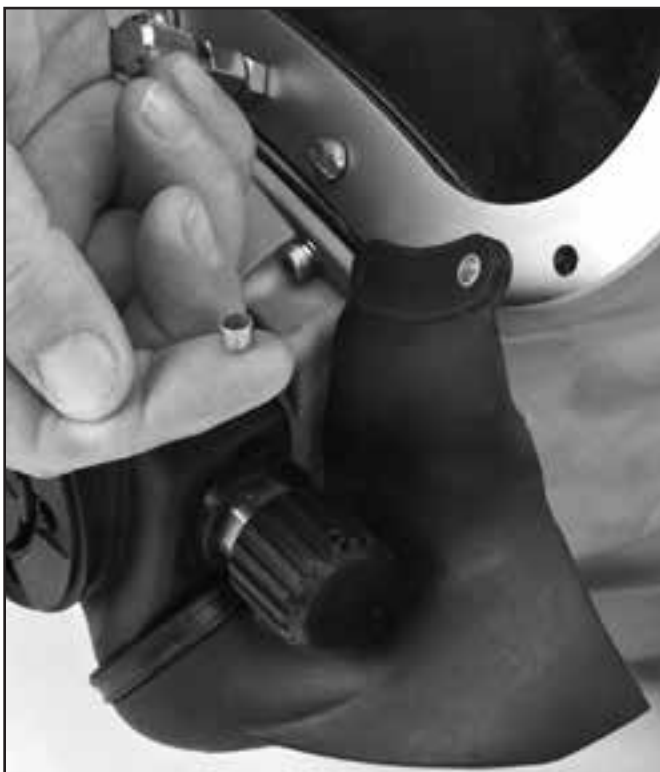
Make sure the whisker spacers are in position before tightening the screws that secure the whiskers.
