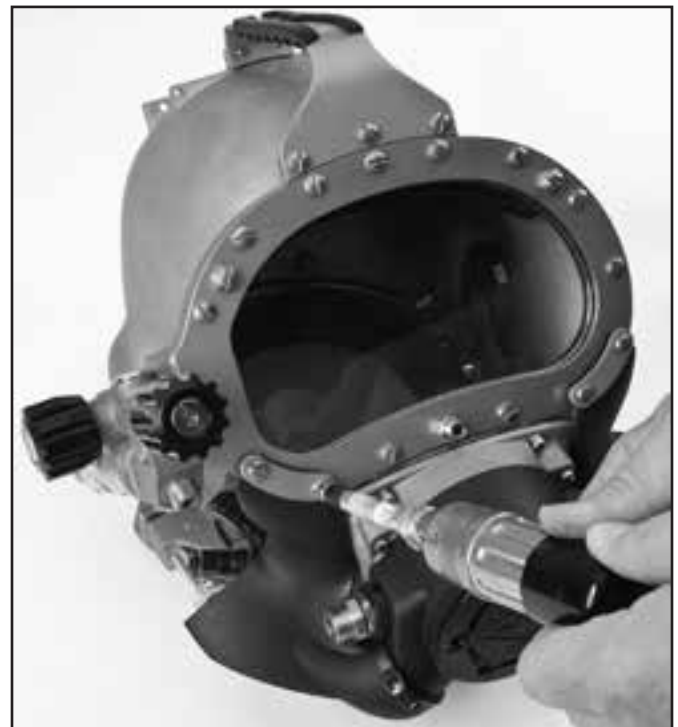
Only use a torque screwdriver to tighten the screws that secure the whiskers to the face port.
