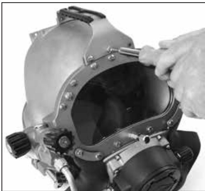
Unscrew the front three handle retainer screws.
