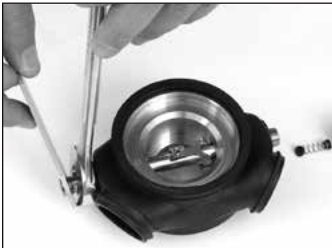
Loosen the nipple tube jam nut to remove the tube.
