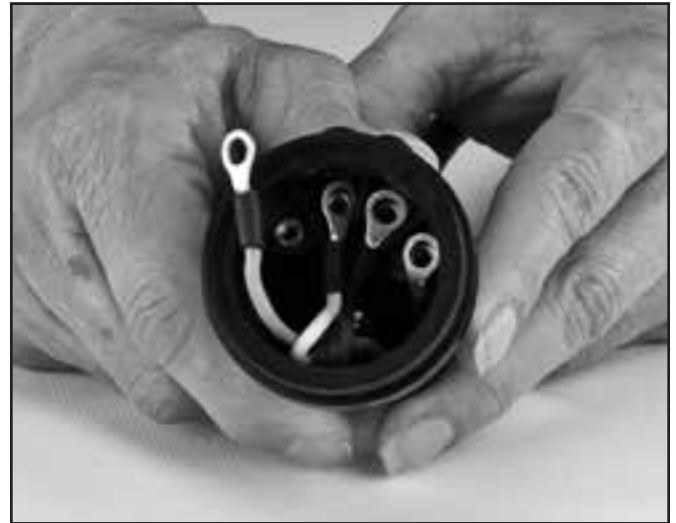
Installing the white wire.
