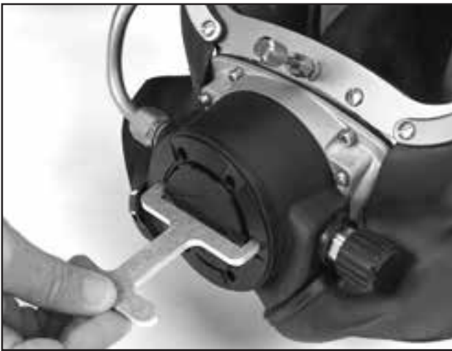
Start removal of the cover by unscrewing the retainer ring.
