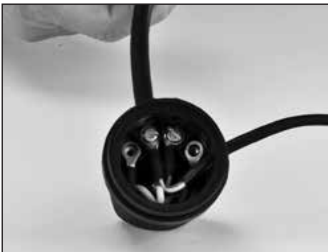
Installing the white microphone wire.
