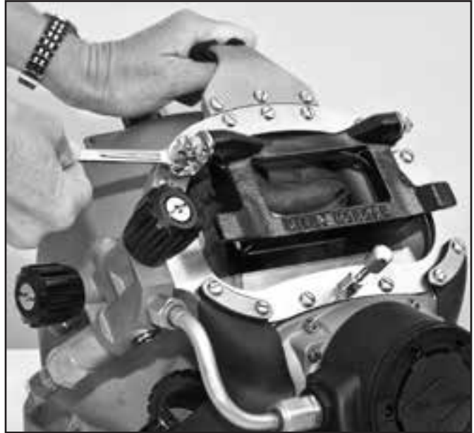
Tighten the weld lens assembly.
