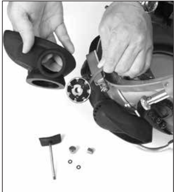
Remove the microphone so you can remove the oral/nasal mask.
