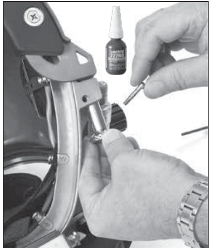
The screws that secure the sealed pulled pins must be properly installed and torqued.
