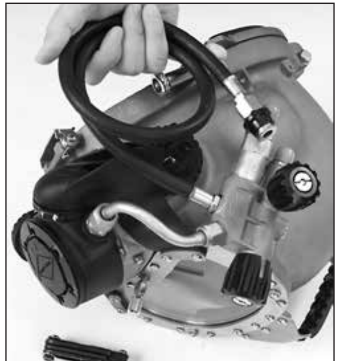
Thread the hose into the side block opening.
