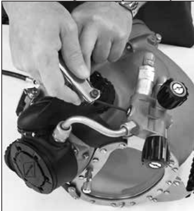
Remove the plug from the side block and install the inflator hose here.
