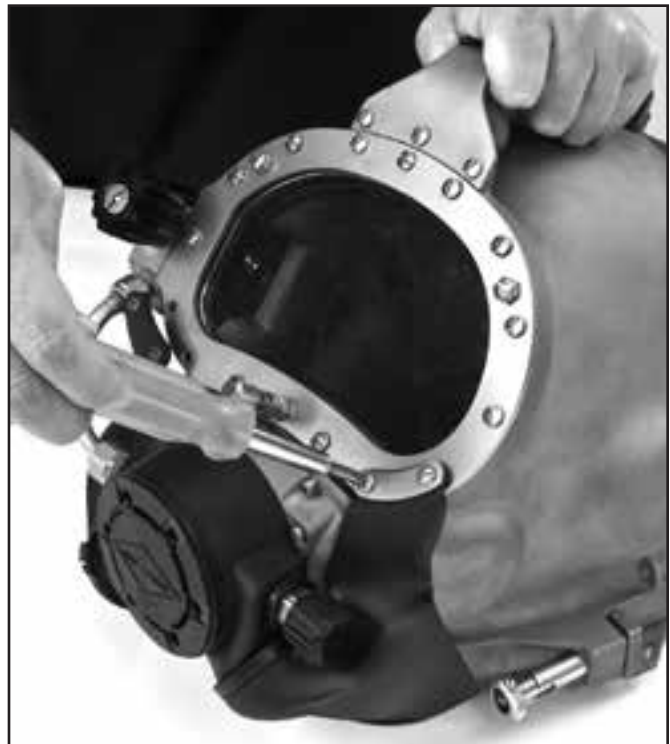
Remove the screws that secure the port retainer.
