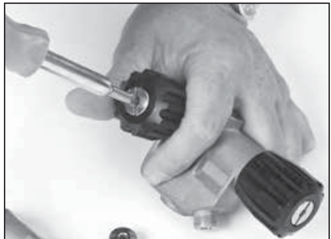
Tighten the nut that holds the handle in place.
