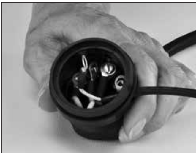
Installing the red microphone wire.
