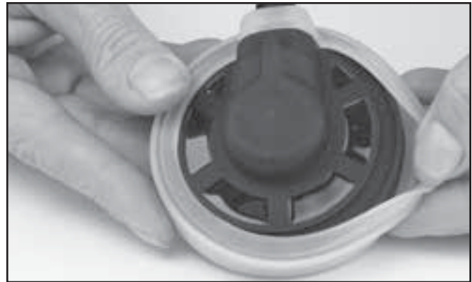
Removing the rubber cover from the earphone.
