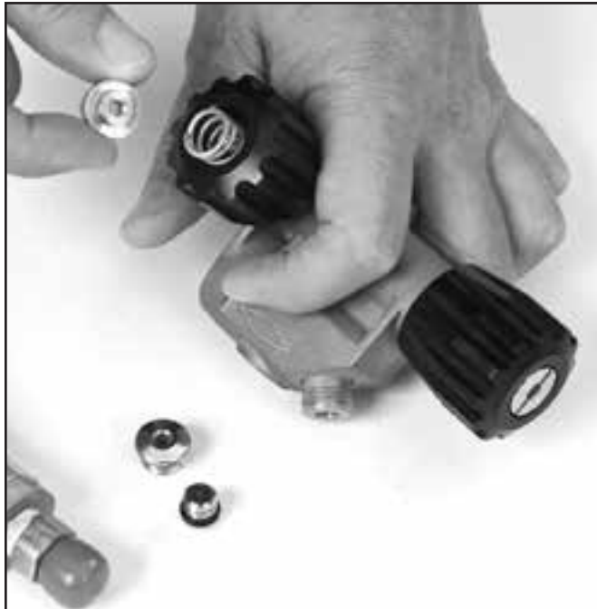
Remove the lock nut and spring
