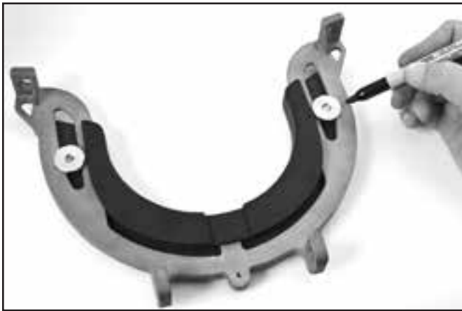
Prior to disassembly of the locking collar, mark the position of the washers.
