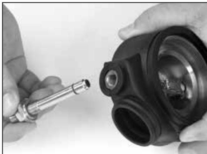
Carefully remove the nipple tube.
