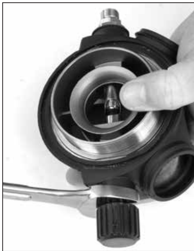
Tighten the packing nut on the adjustment knob.
