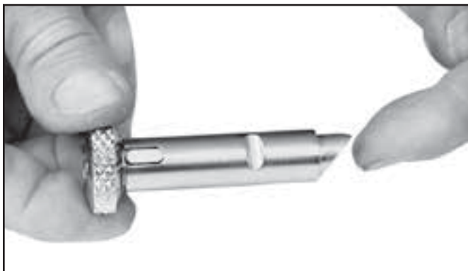
The cam angle must be correct for the pins to work properly.
