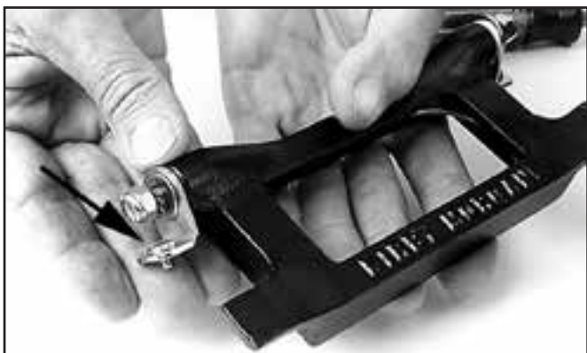
Install the screws through the mount ears.
