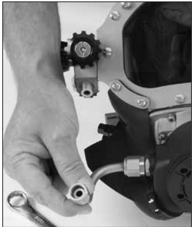
Swing the bent tube down and out of the way.
