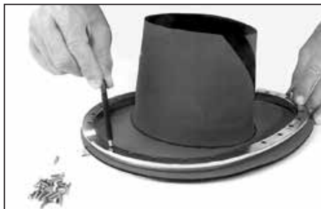
Use a small, sharp punch to locate the bottom hole.
