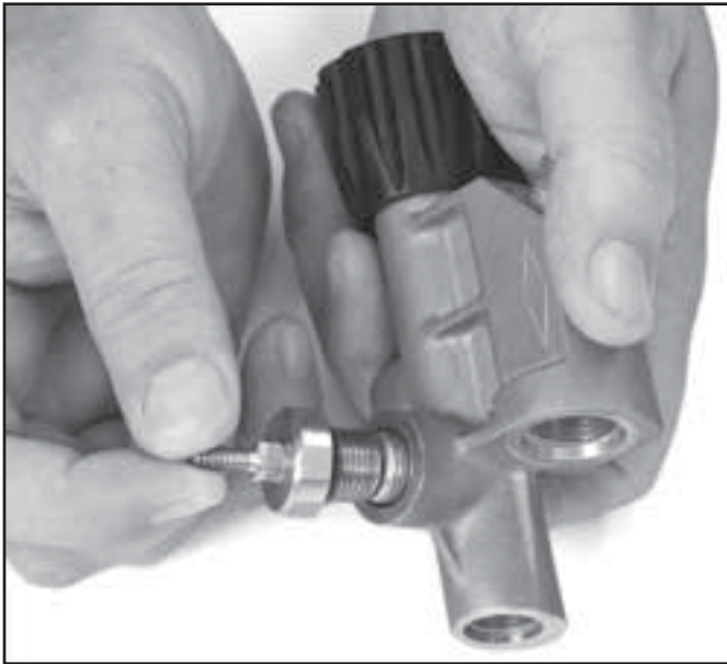
The valve stem must engage the seat properly.
