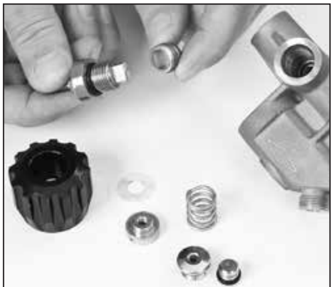
Removal of the bonnet, valve stem, and seat.
