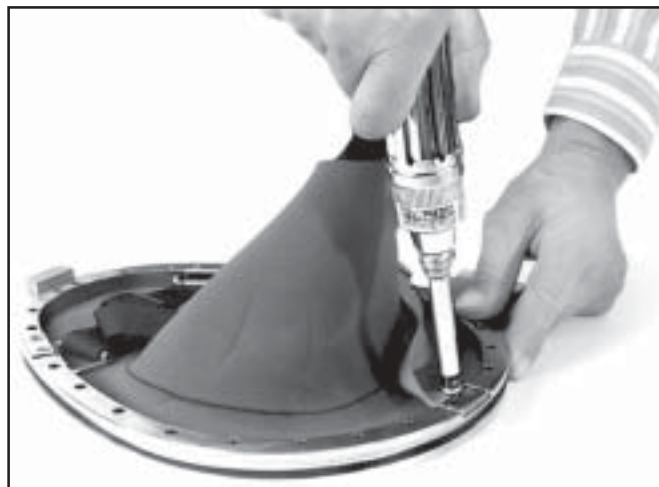
Tighten all the screws to 14 inch pounds (16 kg.cm.) of torque.
