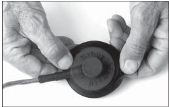
Removing the rubber cover from the earphone.
