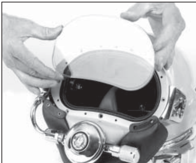
Place the new face port into the helmet shell
