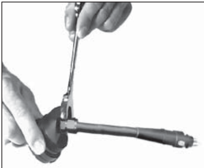
Use a 3/4 inch wrench to unscrew the waterproof connector.
