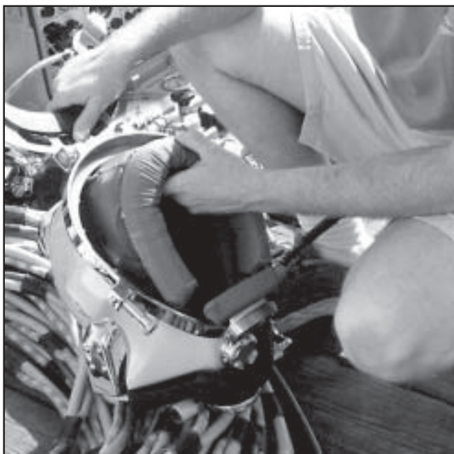
The head and chin cushions are easily removed.
