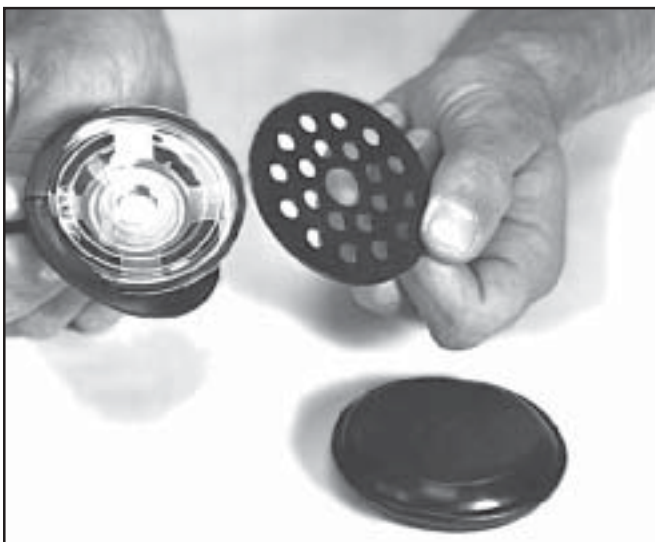
Fig. 5.5 Uncover the earphones so they may dry.
