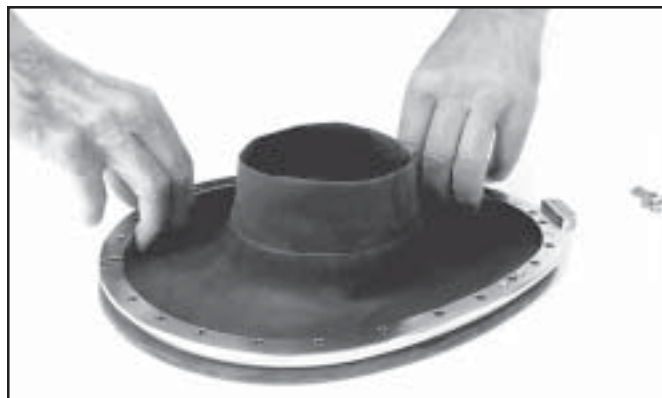
Center the split rings by pressing on the dam and feeling the inside edge of the stepped ring and the split rings.
