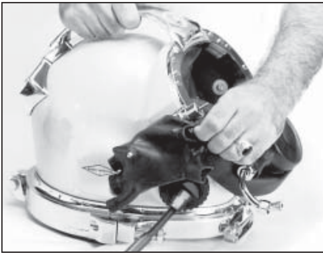
Position the shroud over the side block.
