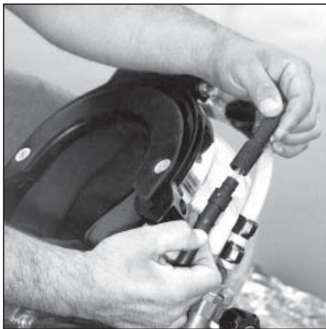
Fig 2.7 - Connecting the waterproof connectors.
