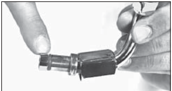
Replace the O-ring on the bent tube if it is worn or damaged.
