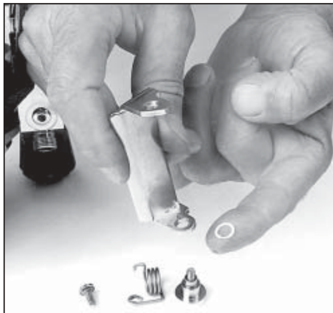
Make sure you have not dislodged the Teflon® washer.
