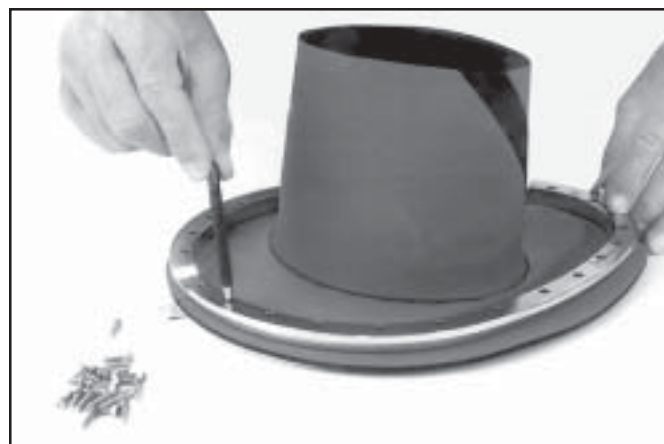
Use a small, sharp punch to locate the bottom hole.
