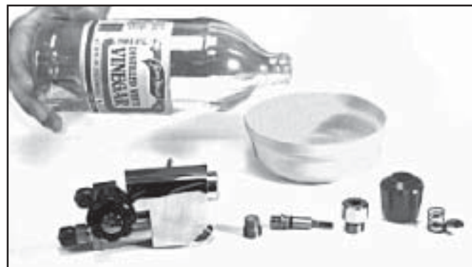
Clean all the metal parts to remove salts.
