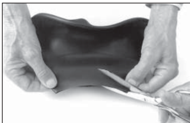
Trim latex neck dams with the largest, sharpest scissors available.
