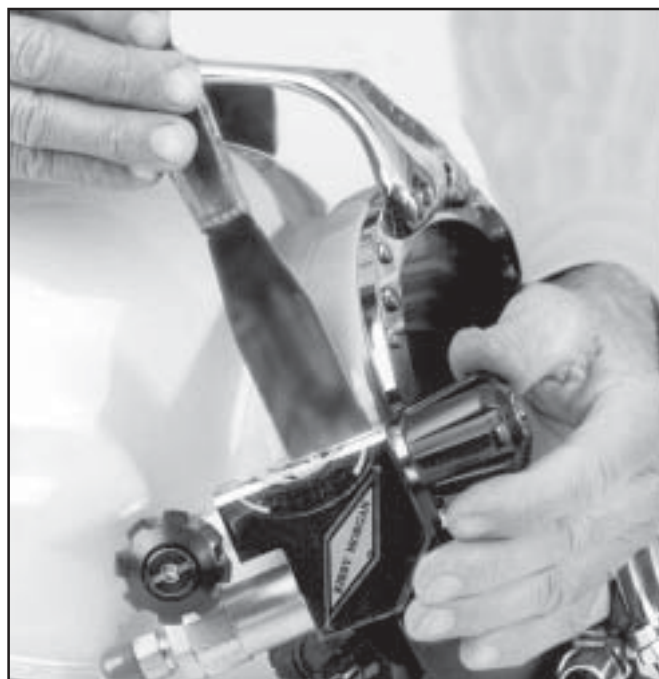
A thin putty knife can be pushed between the side block and the helmet shell
