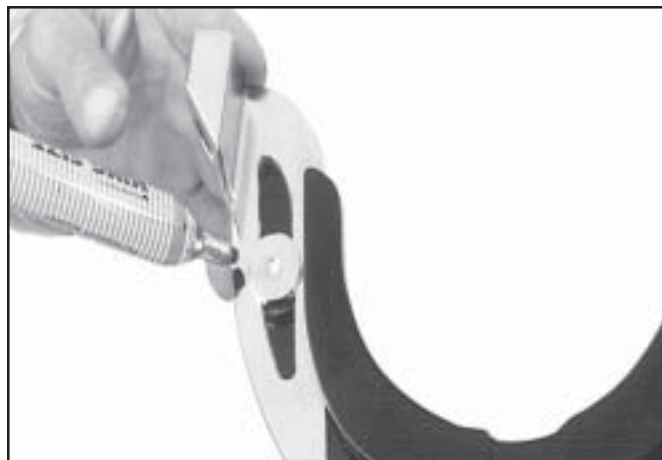
Prior to disassembly of the locking collar, mark the position of the washers.
