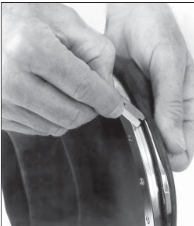
Use a sharp razor blade to trim the excess latex.
