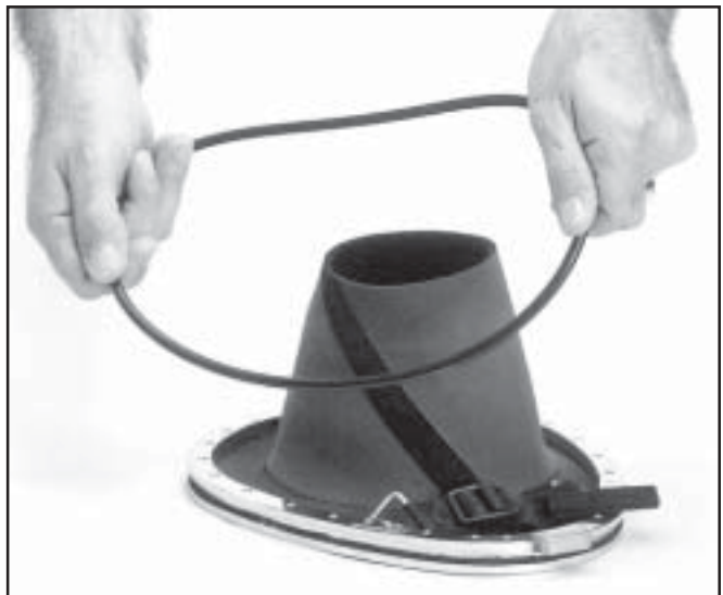
Inspect the O-ring on the neck dam.
