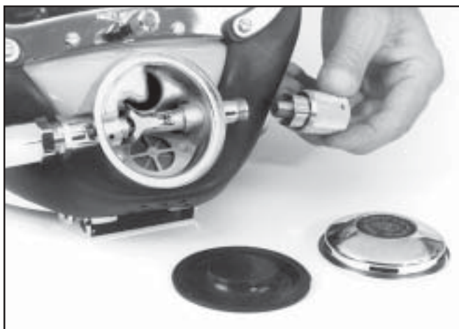
Fig. 6.23 - Screw the regulator adjustment knob out for removal.
