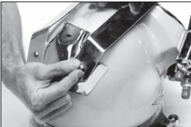
Reinstall the two rear weight screws and washers
