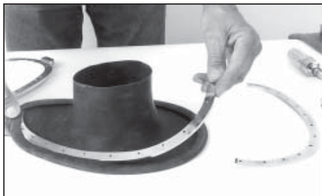
Install the split rings inside the trimmed outer lip of the neck dam.
