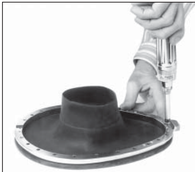
Use the screw to punch through the neck dam.
